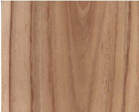
**Above:** The wood can be kiln dried, with only a 2.5% radial and 8.5% tangential loss of volume.
